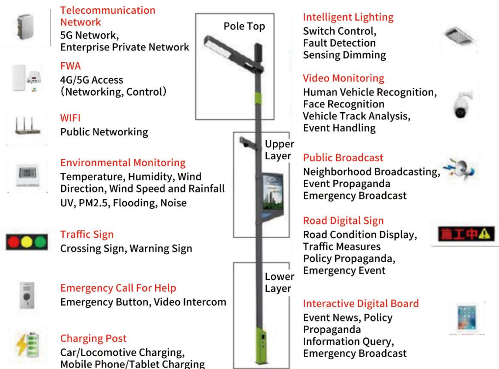
Figure 4.2-2 Schematic Diagram of 5G Smart Pole Mounting Device (Quoted from the "Smart Pole Technical Specifications and Verification Industry Cooperation" of the Institute for Information Industry) [17]
