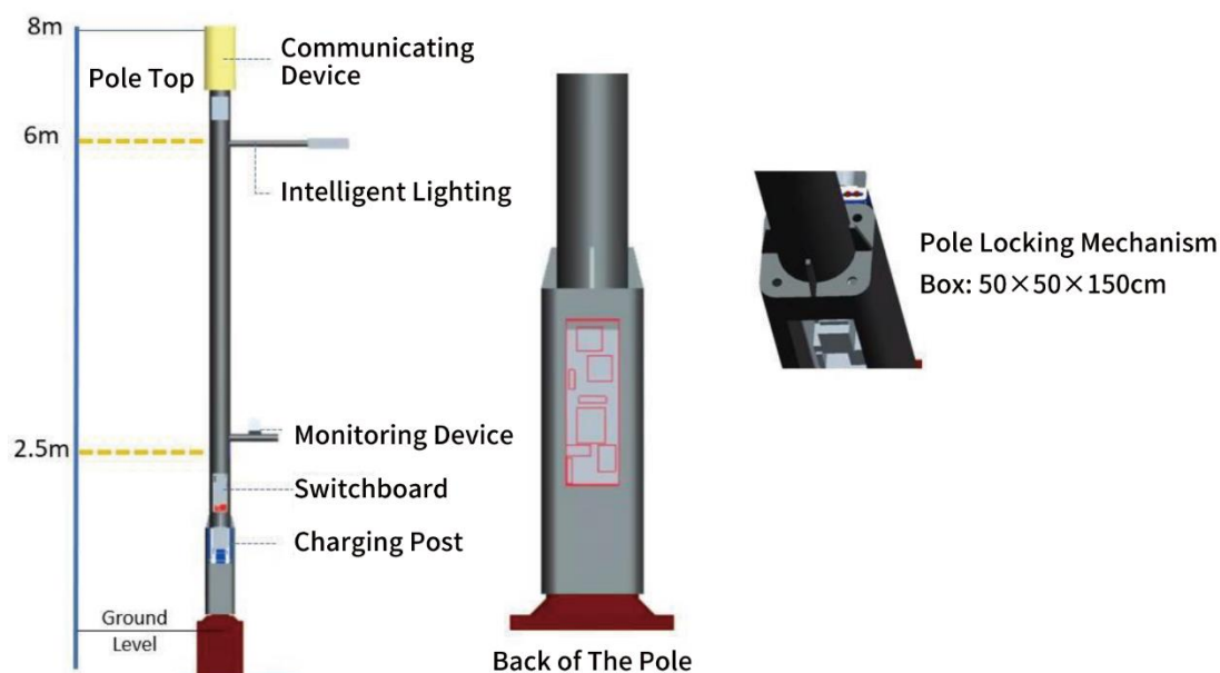
Figure 4.5.2.1-1 Type 4 Smart Pole Mounting Intention
